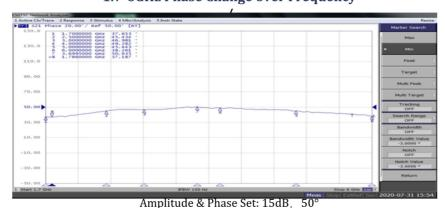
Phase tested (Max: 50.635° Min: 37.187° Max-Min: 13.448°)
